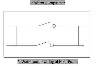
Note: The installer should connect 1 parallel with 2 (as above picture). To start the water pump, condition 1 or 2 is connected. To stop the water pump, both 1 and 2 should be disconnected.
