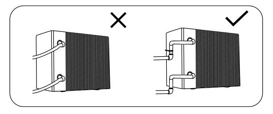
DO NOT install water pipes in a way that they pass behind the heat pump's evaporator. In case this cannot be avoided, cover the pipes with thermal insulation foam.
