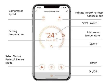
2. For heat pump with Heating & Cooling function:
